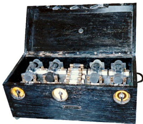
Four valve amplifier made by Radio Apparat Gesellschaft mBH with four type Siemens A valves.
