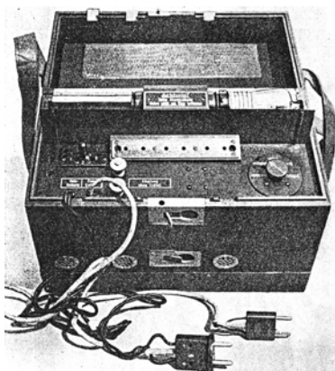
Amplifier and circuit diagram with two Siemens & Halske Type SS I space charge valves.
