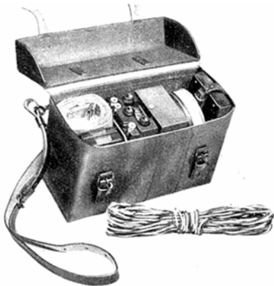
The DLE (kl.) with the battery box and spare parts was packed for transport in a leather bag.
