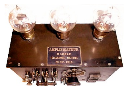
Top view of desk model 3 ter amplifier.
