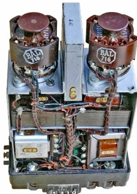
The DLE (kl.) amplifier detached from its cover, as seen from the bottom, revealing the two RV 2.4 P 45 valves in their holders.
