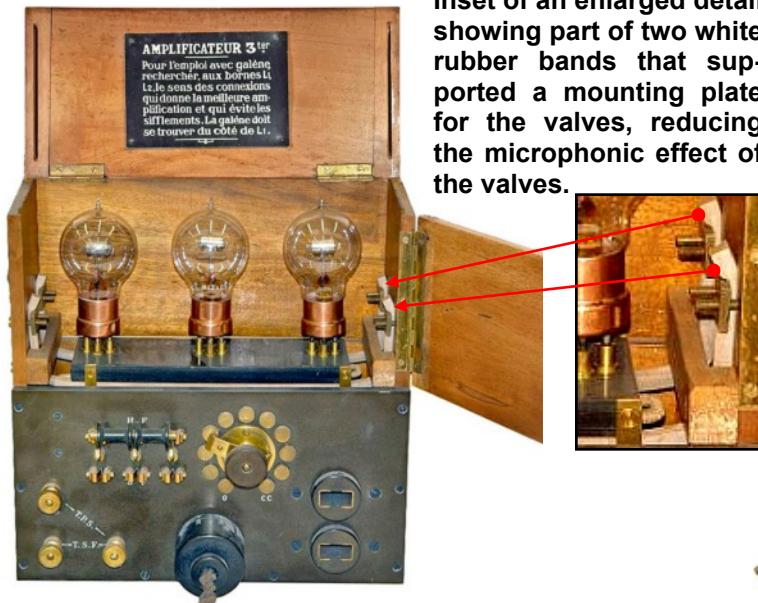
French 'Amplificateur 3 ter ' with the hinged top and front door open, revealing the three TM valves.
